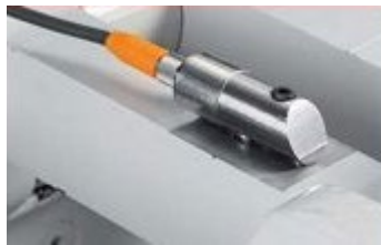
Fig.1 - Machine closing force detection sensor
